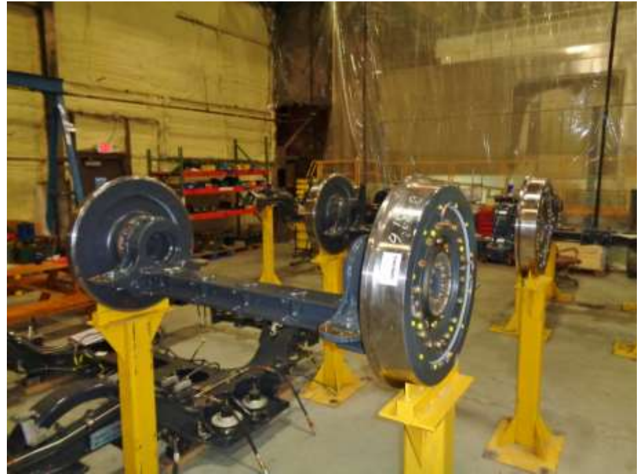
Wheel-sets attached to the truck frame
