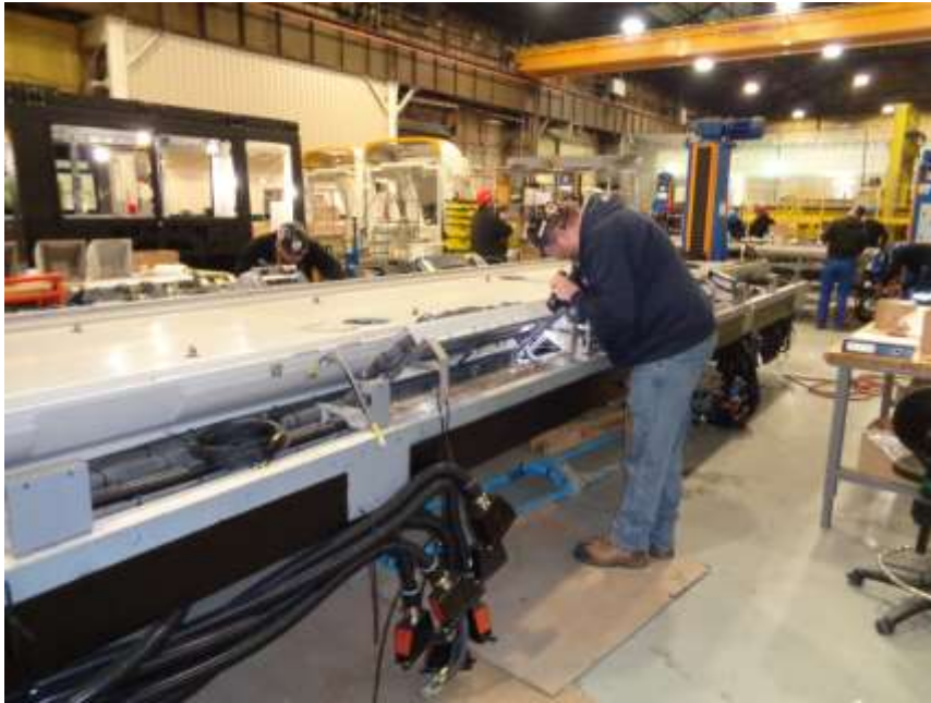
Worker wires the roof section
