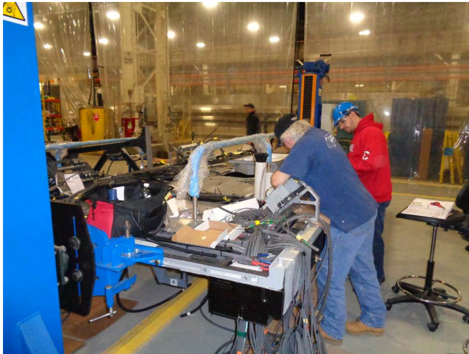
Photo 234: Wiring the ceiling of the roof panel with it flipped over in the assembly jig
