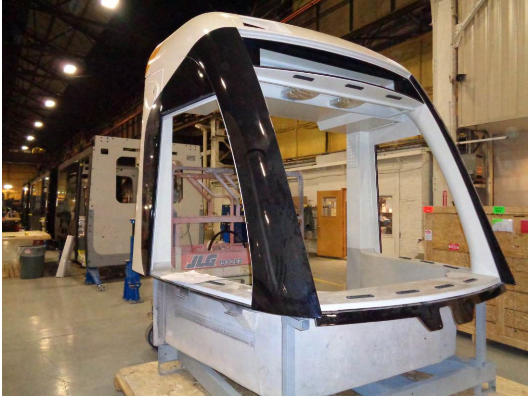
Photo 25: Streetcar cab fairing, installed over a structural frame
