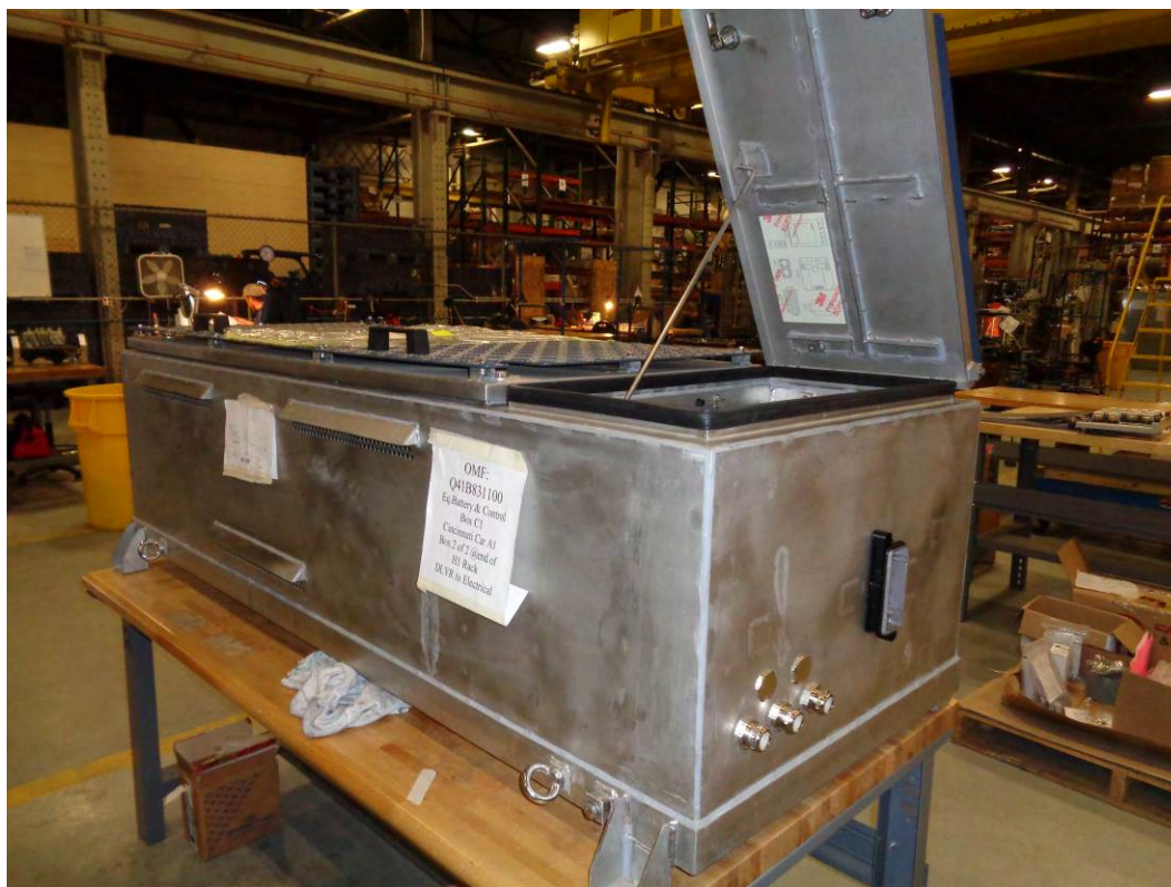
Photo 24: Auxiliary battery and control box prior to mounting on the roof panel
