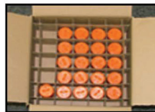
CORRECT (Protective caps in place)
