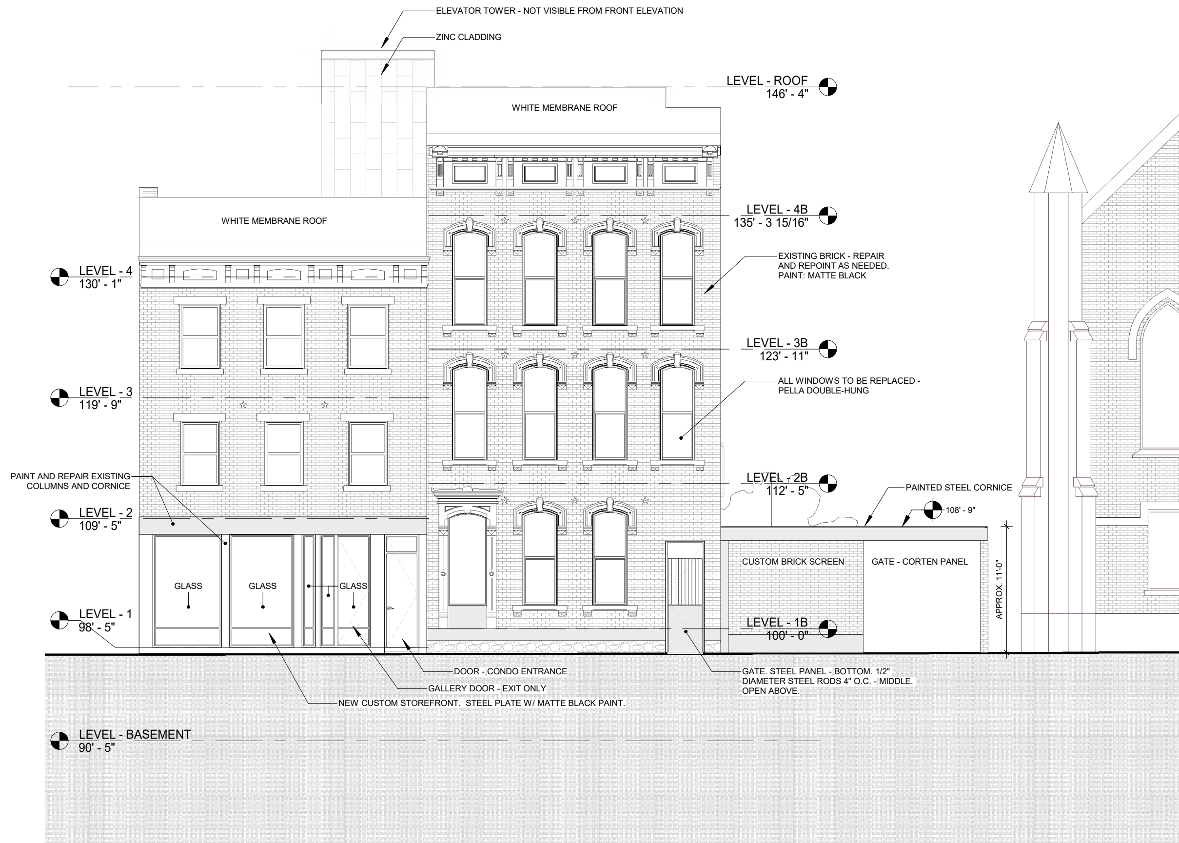
1 ELEVATION - WEST (FRONT) PROPOSED 1/8" = 1'-0" VIEW REFERENCED ON: A105- 1
