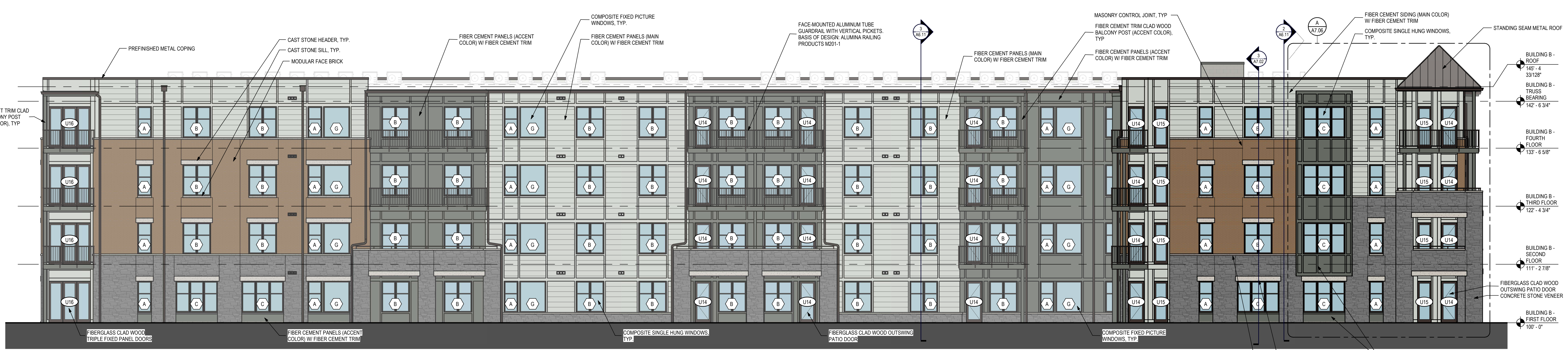
2 building b - south elevation A6.03 1/8" = 1'-0"
