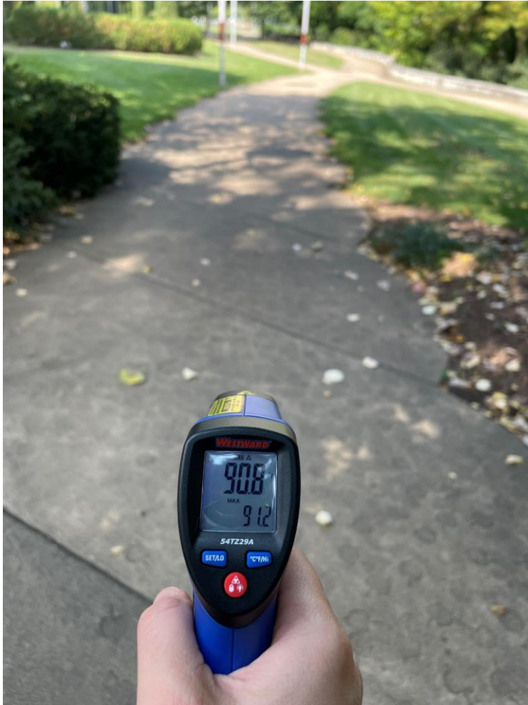
Surface temperature of the walking path at TM Berry Friendship Park in an area shaded by trees on 8/25/23 when ambient temperature was 95 F.
