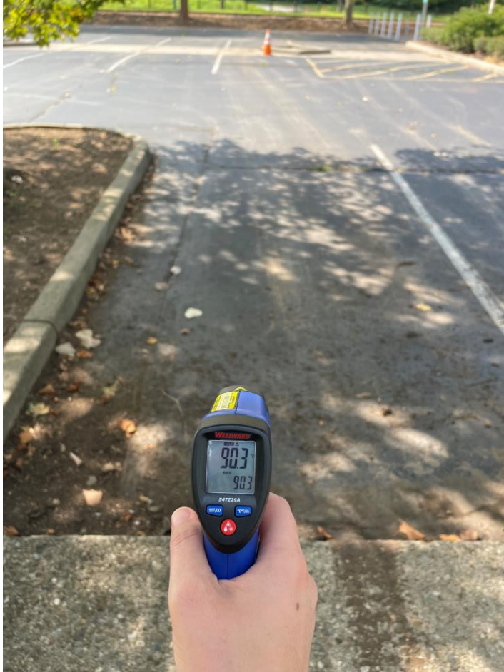
Surface temperature of the parking lot at TM Berry Friendship Park parking lot in an area shaded by trees on 8/25/23 when ambient temperature was 95 F.
