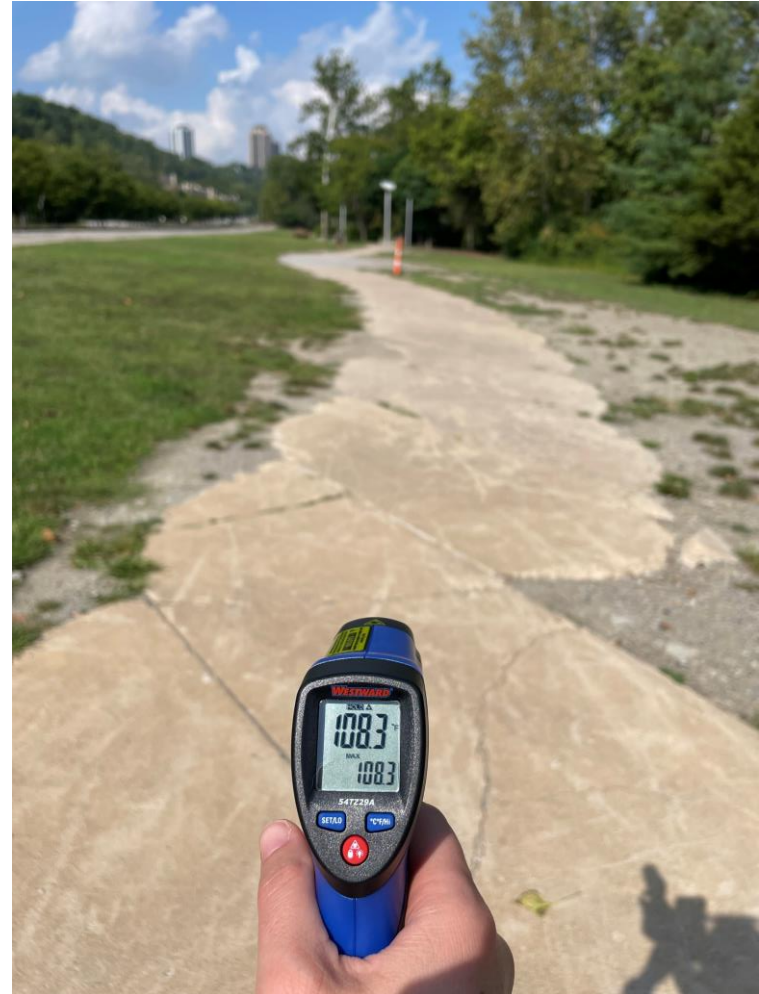
Surface temperature of the walking path at TM Berry Friendship Park in an area without tree cover on 8/25/23 when ambient temperature was 95 F.
