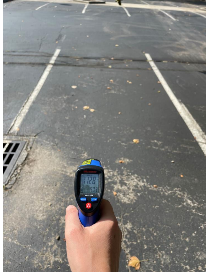
Surface temperature of the parking lot at TM Berry Friendship Park in an area without tree cover on 8/25/23 when ambient temperature was 95 F.
