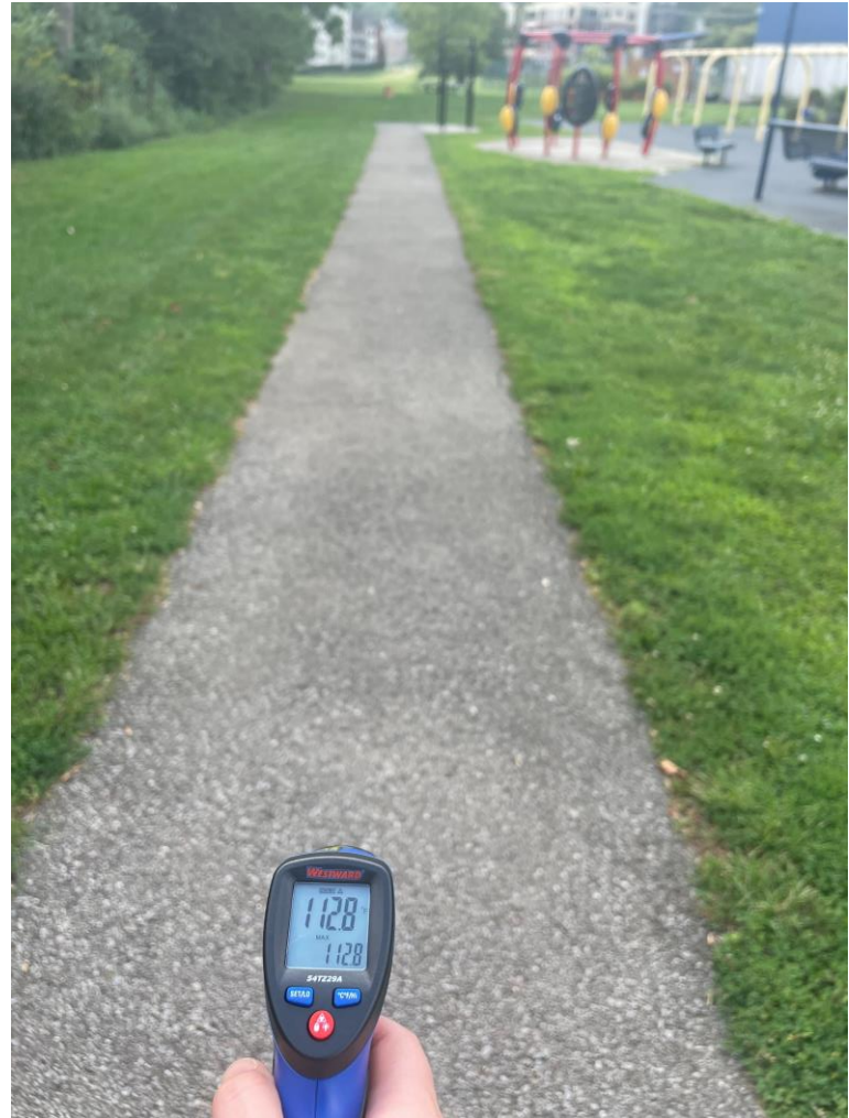
Surface temperature of the walking path at LeBlond Recreation Center on 8/25/23 when ambient temperature was 95 F.
