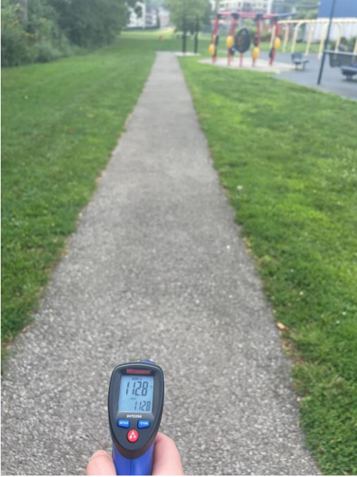
Surface temperatures of various materials at LeBlond Recreation Center on 8/25/23 when ambient temperature was 95 F.
