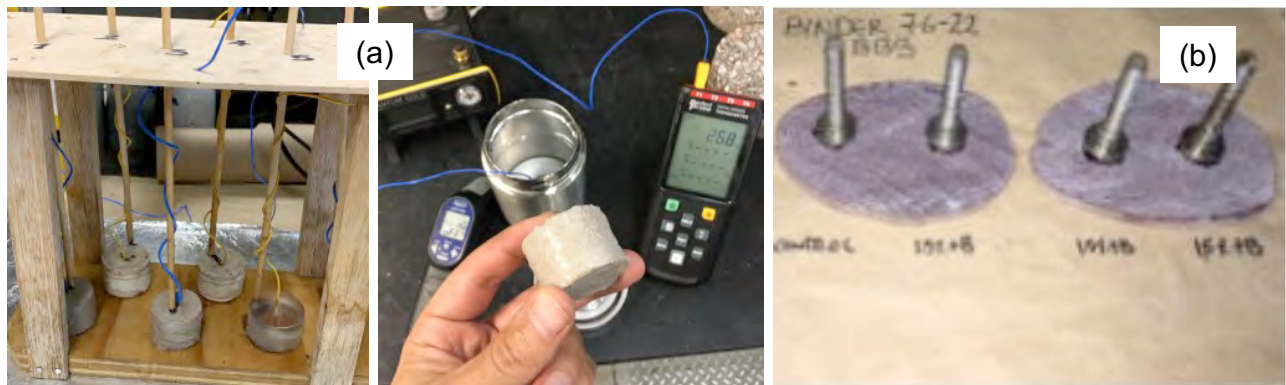
Figure 13: a) Thermal conductivity test setup; b) Bitumen bond strength test setup.
