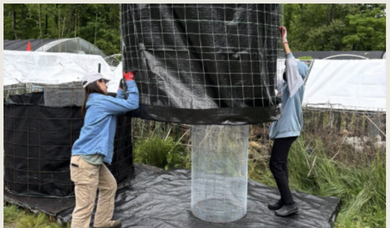
Figure 9A: Placing outer chimney around inner chimney
