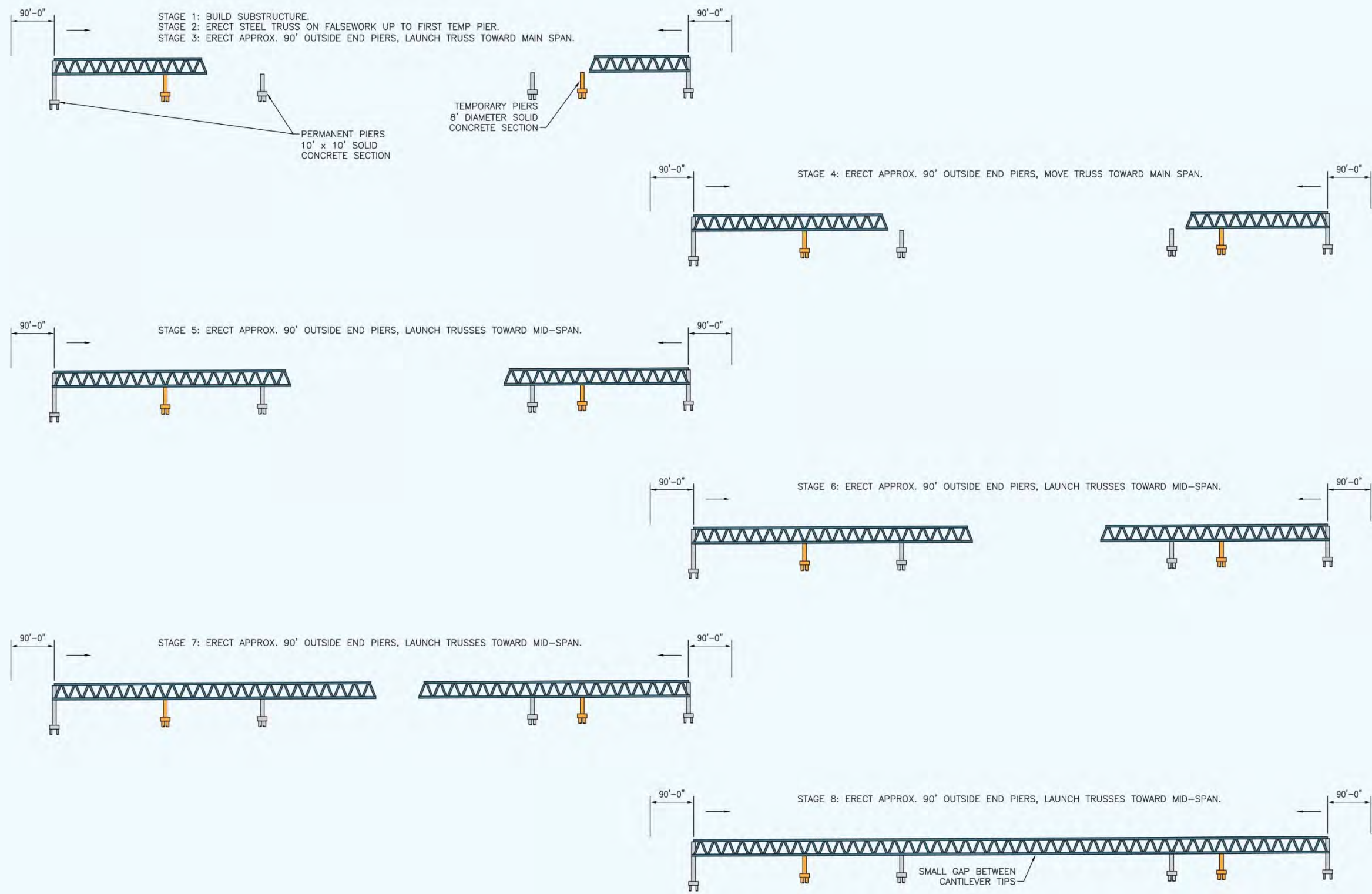
Long Span Push Launch Construction Method 4 of 5
