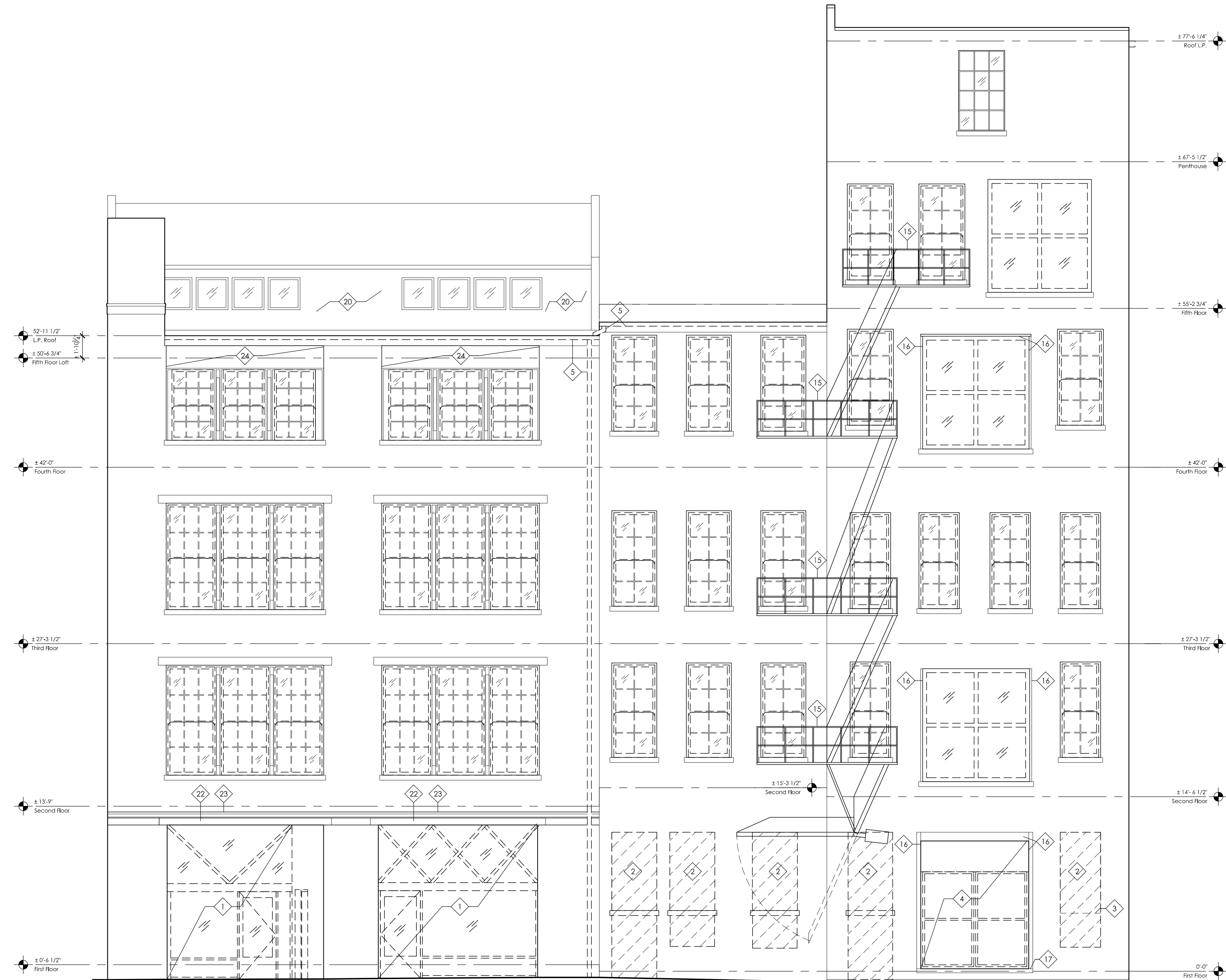
1 A5.0 DEMOLITION EAST EXTERIOR ELEVATION 3/16" = 1'-0"
