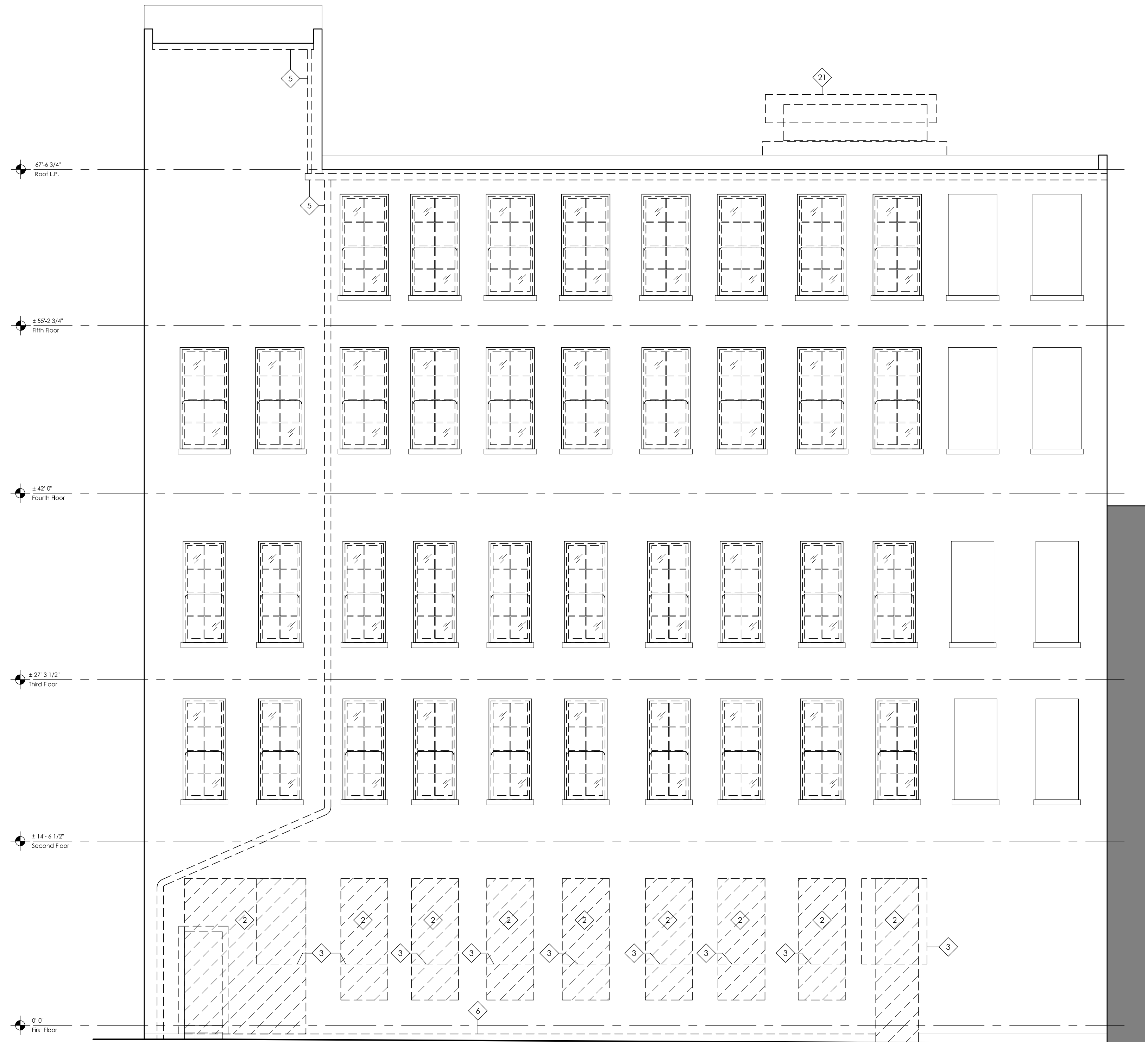
1 A5.1 DEMOLITION NORTH EXTERIOR ELEVATION 3/16" = 1'-0"
