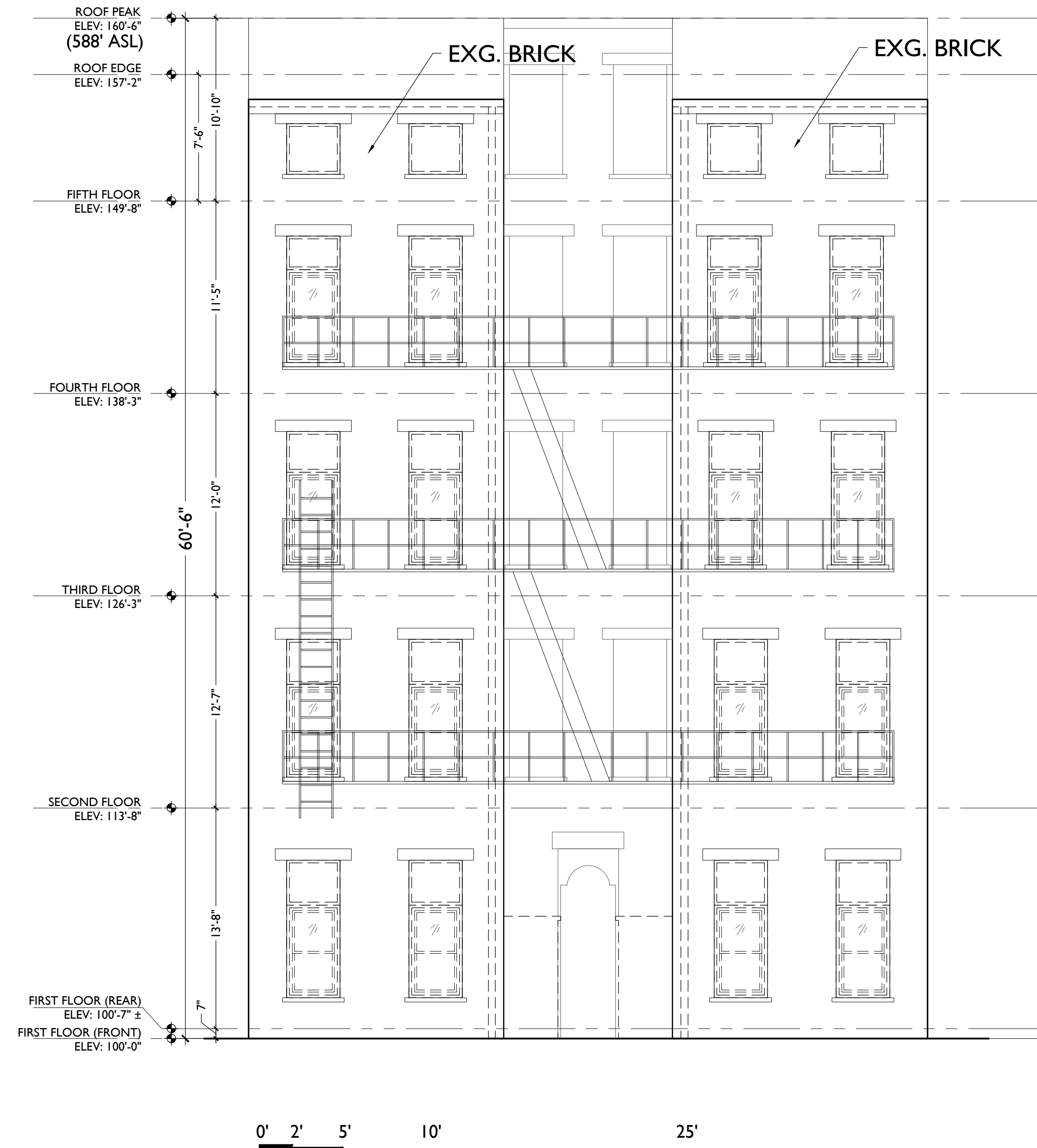
SCALE: 3/16" = 1'-0" DEMOLITION EAST ELEVATION 2
