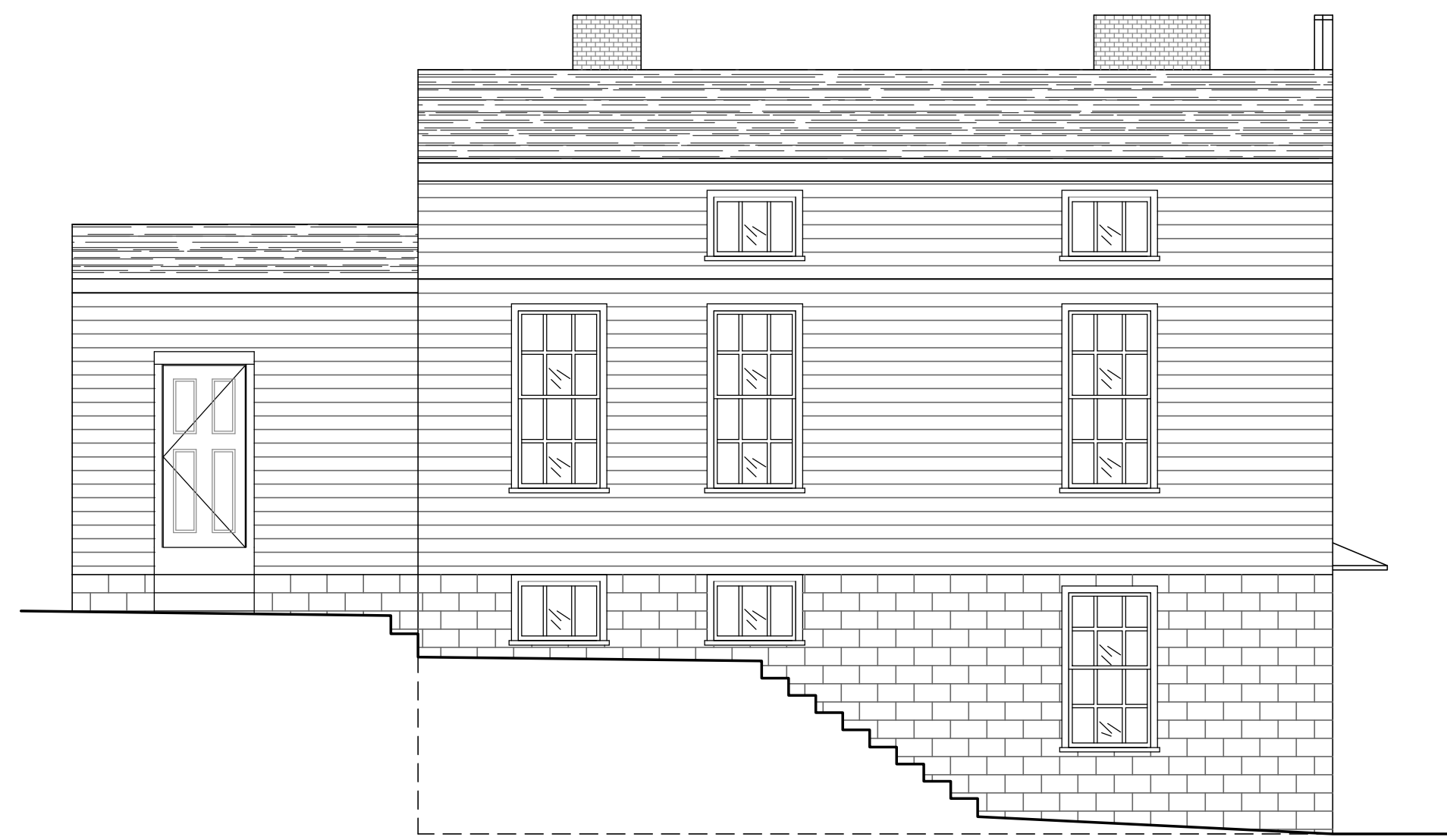
4 WEST ELEVATION - EXISTING Scale: 3/16" = 1'-0" 0 2' 4' 8' 16'
