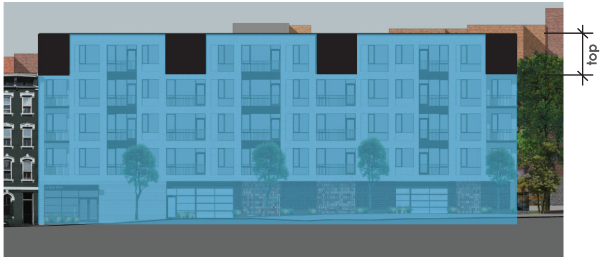
Large single volume broken down by introducing dark material to imply voids along top floor, relating to gaps and voids between smaller scale residential buildings.
