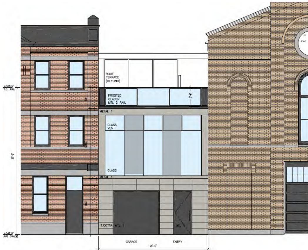
Figure 4: Proposal of permanent tinting 2 of the 5 panels to create a reference to punched openings.
