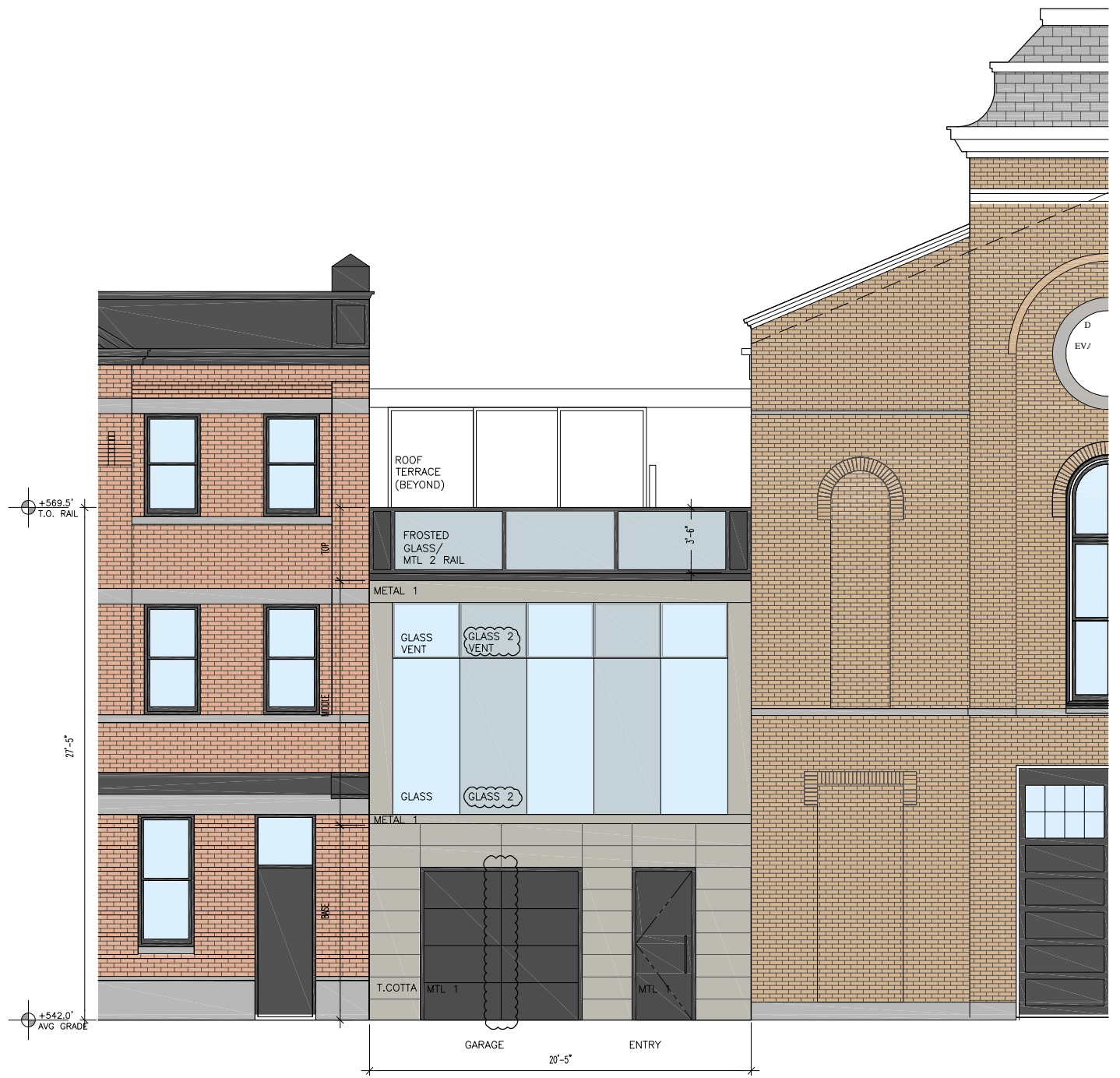
3 West Elevation- Republic Street 1/4"=1'-0"
