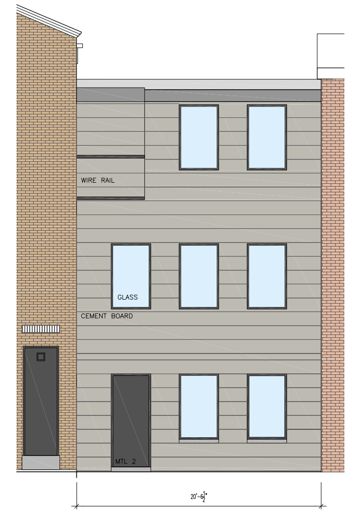
2 East Elevation- Parvis Alley 1/4"=1'-0"
