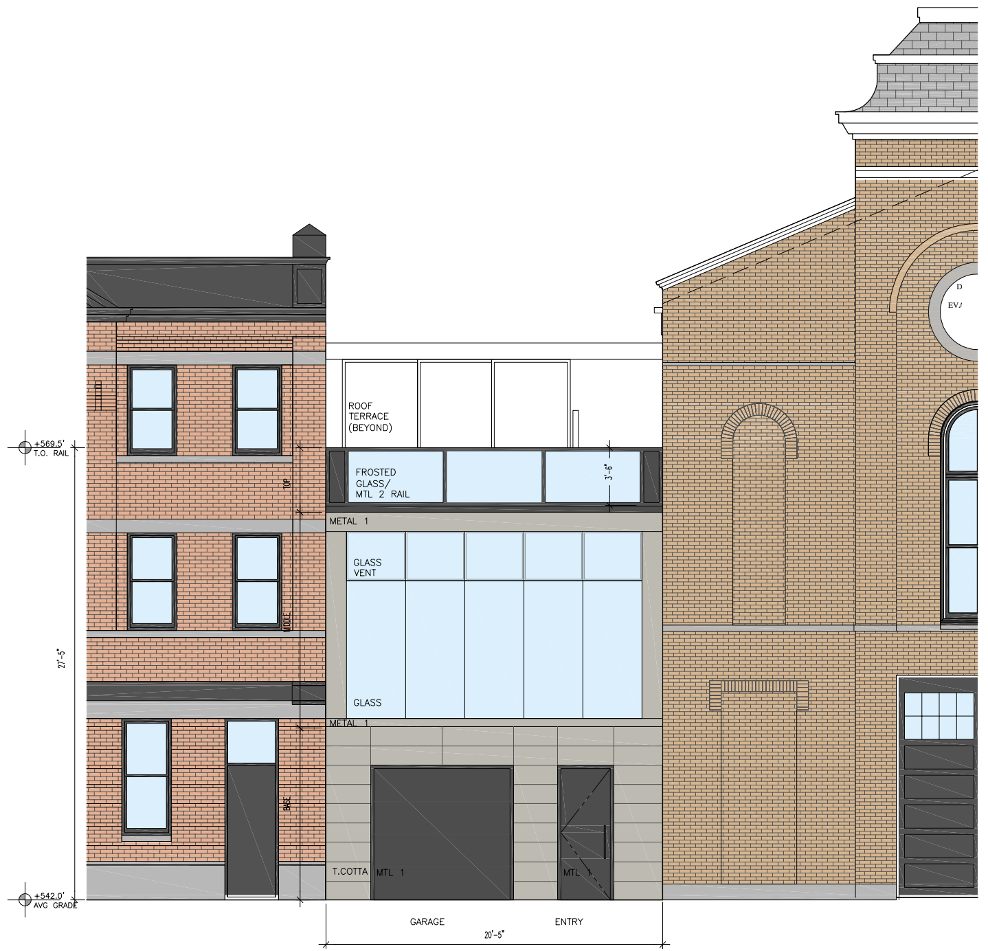
3 West Elevation- Republic Street 1/4"=1'-0"
