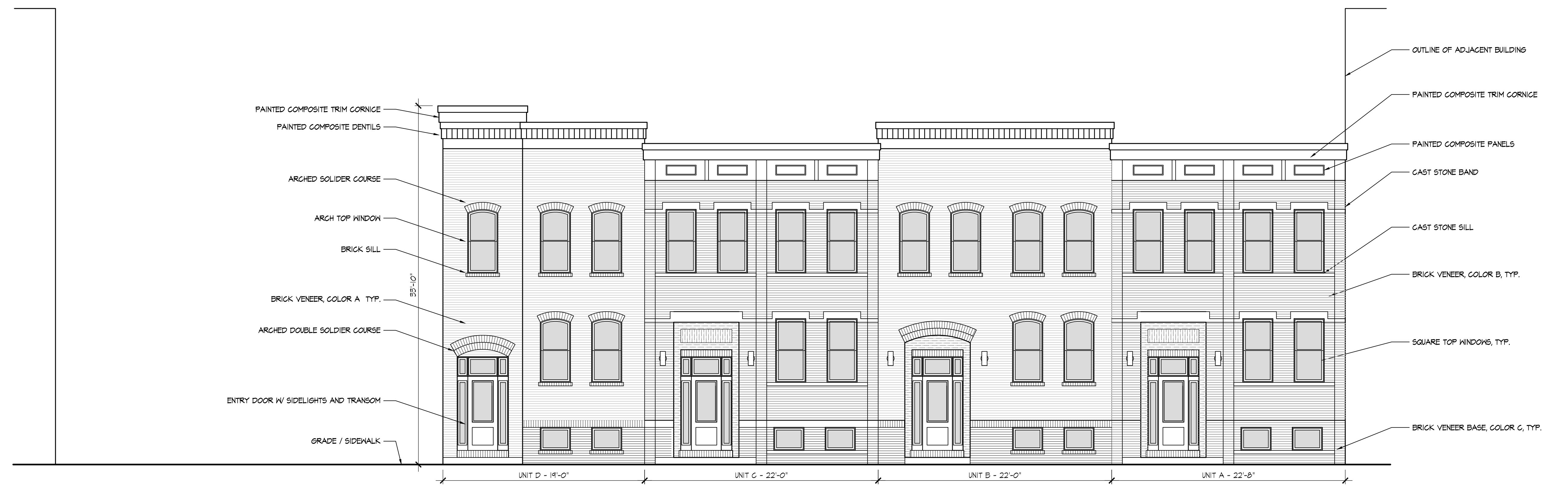
A PLEASANT STREET [FRONT/WEST] ELEVATION SCALE: 3/16" = 1'-0"
