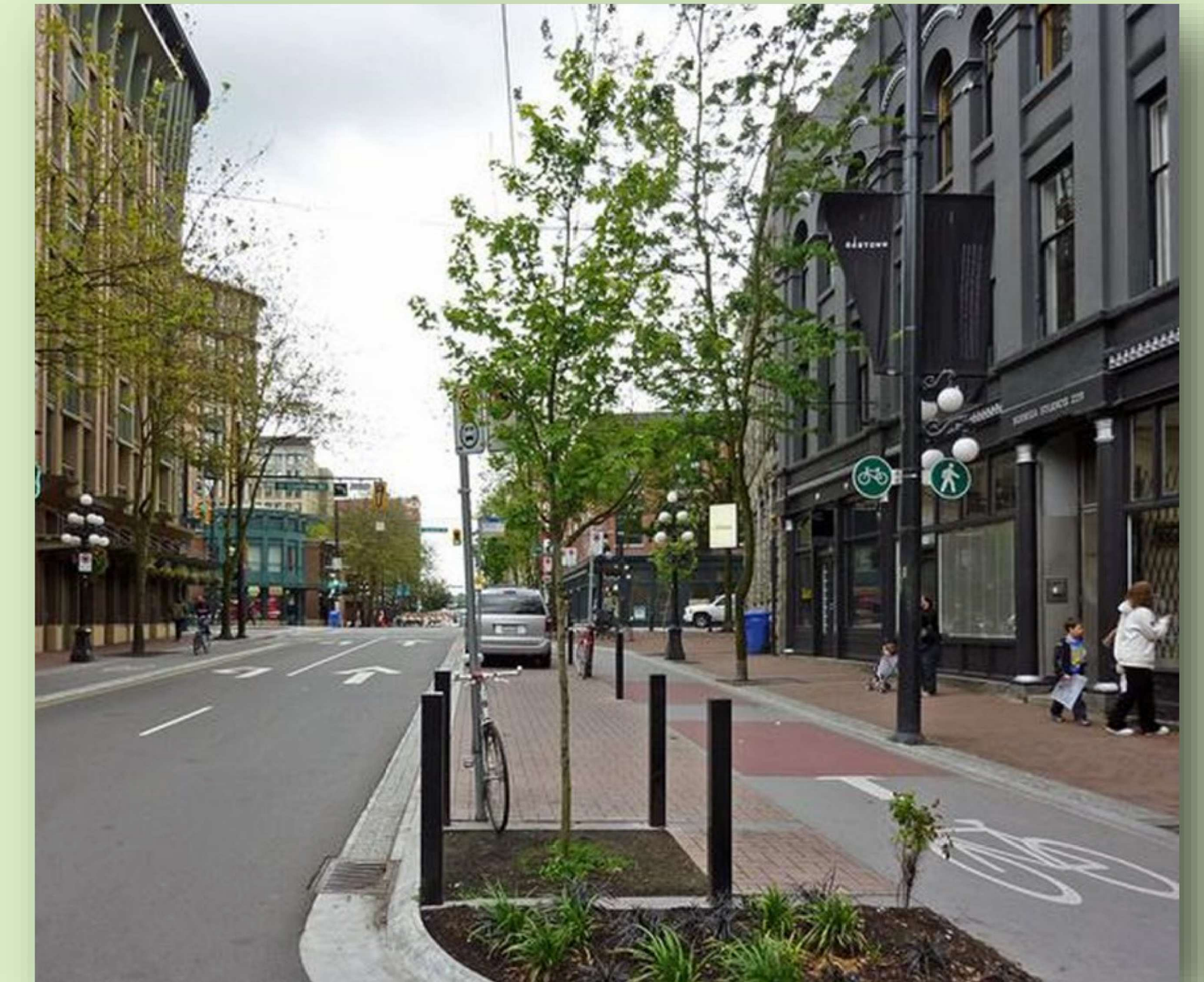
Raised Bike Lane
