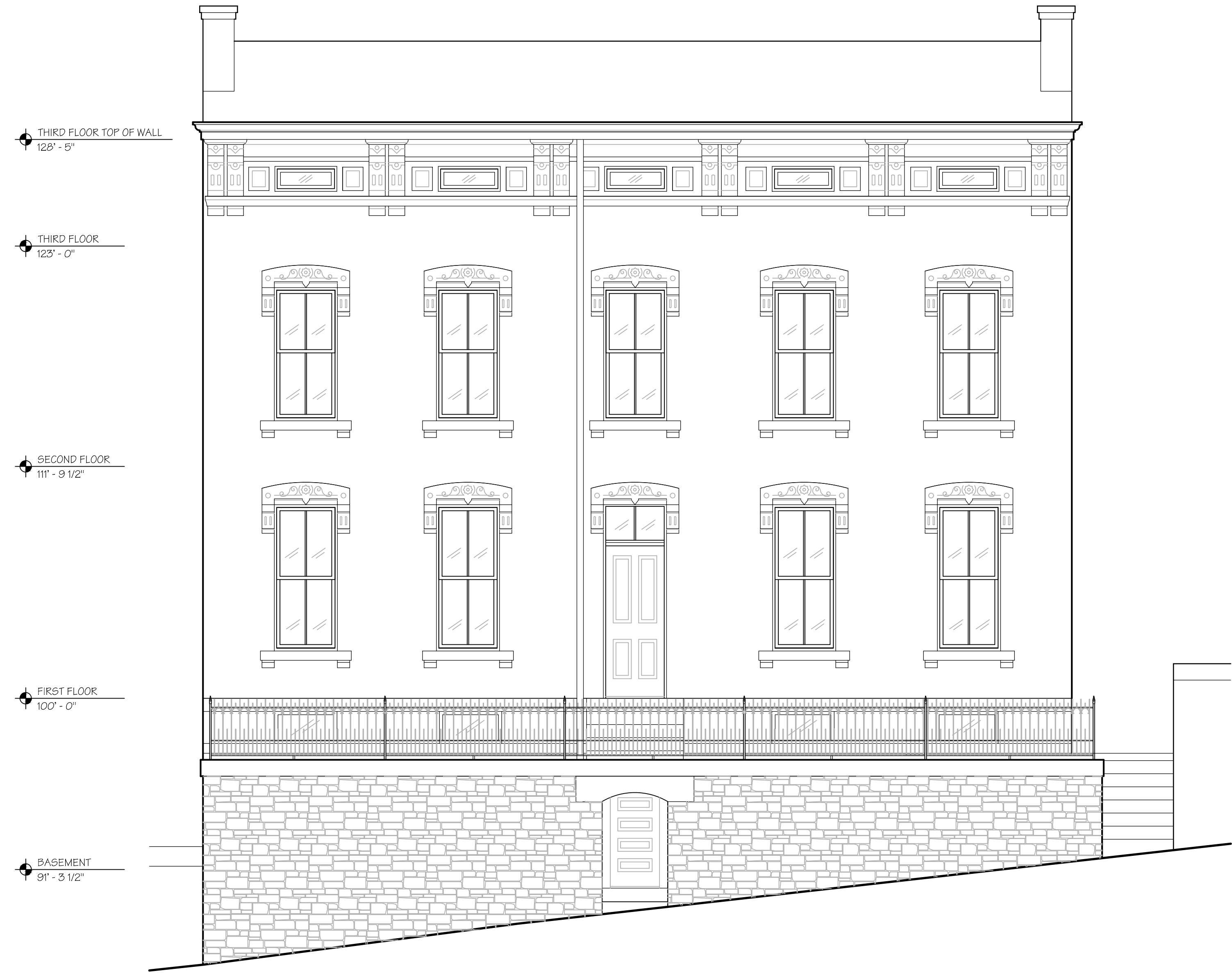
1 South Elevation - Existing A1.2 SCALE: 1/4" = 1'-0"
